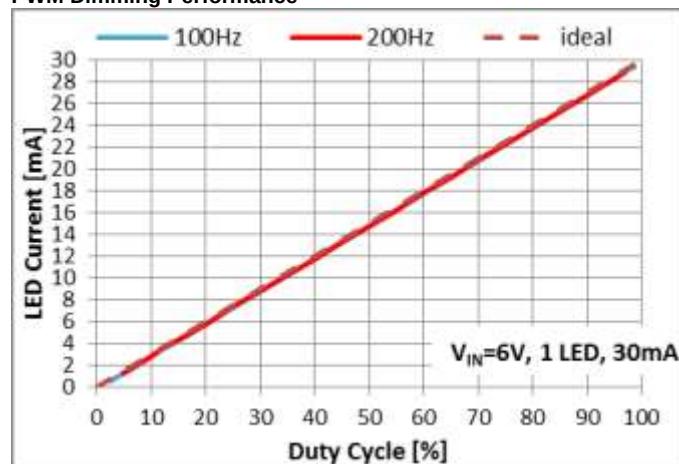
Figure 8 PWM Dimming 30mA vs. Duty Cycle
